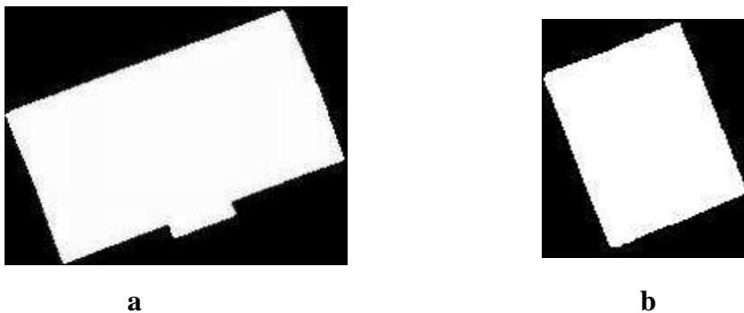
Figure 4: Building class after morphological operation and area threshold
